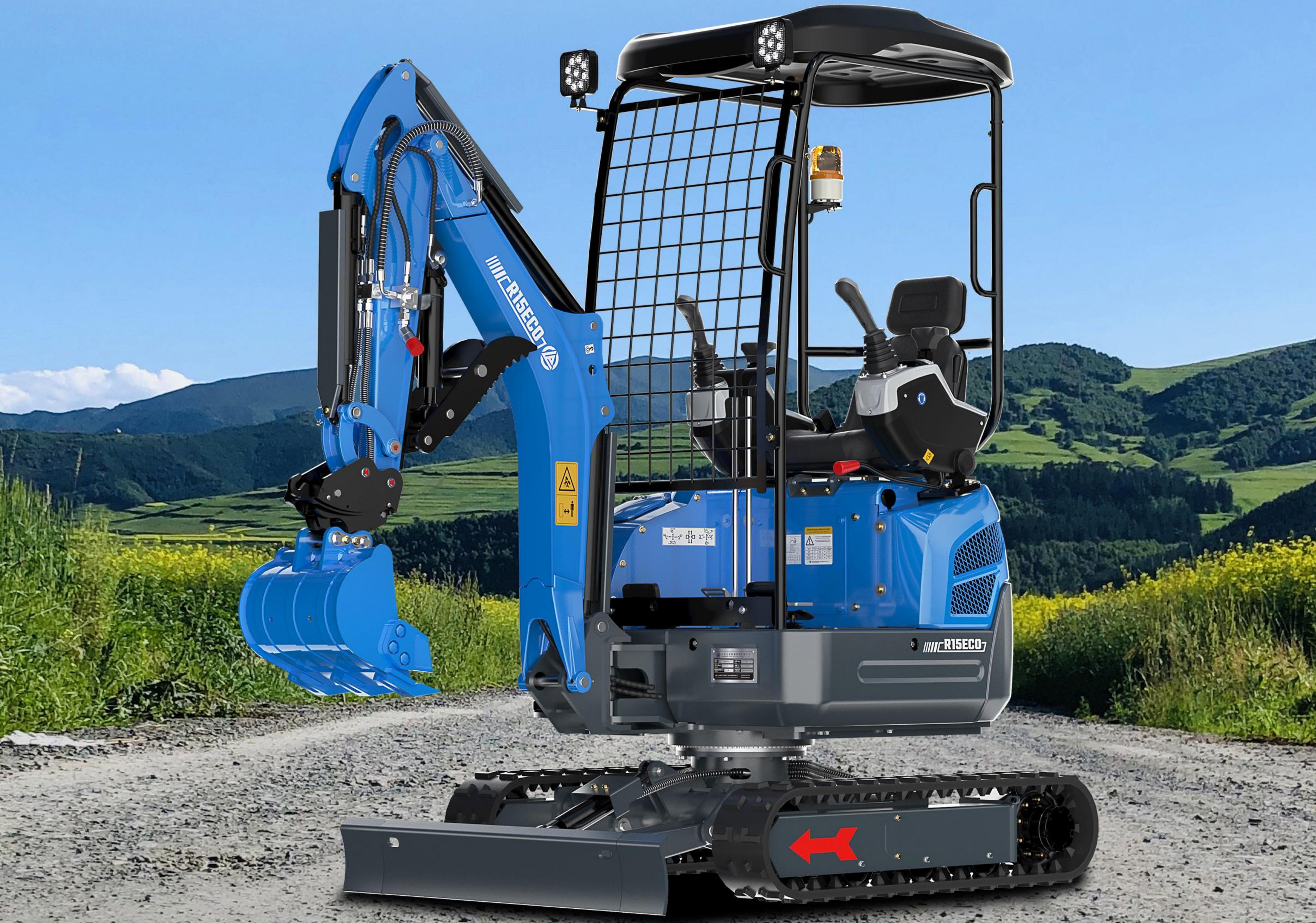
Note: The hydraulic thumb clamp and hydraulic quick change in the figure are optional models. The standard model does not have hydraulic thumb clamp and hydraulic quick change.
