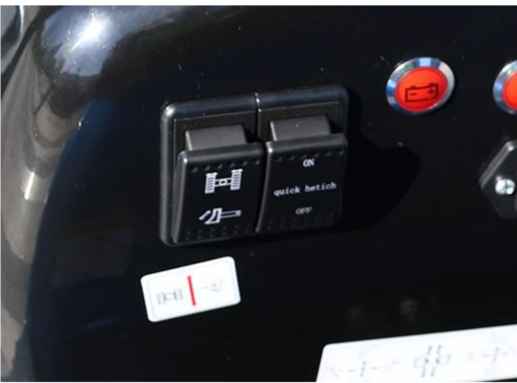
9 Multi-function button The crawler extension and dozer blade switching functions can be realized through simple button operation, as well as the quick change of attachments.
