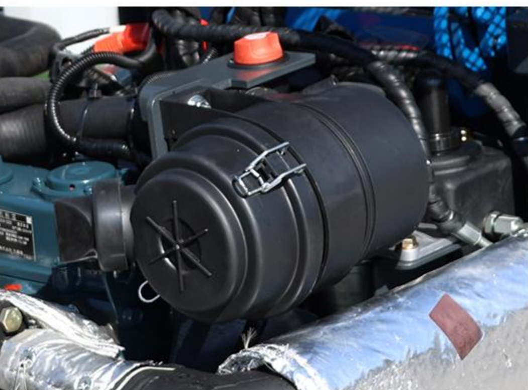
7 Air Filter Prevent dust and impurities from entering the engine's air intake system, thus extending the engine's service life.
